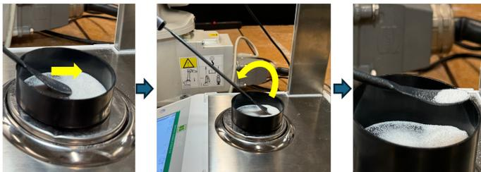
**FIGURE 6:** The figure illustrates the robot executing a predefined scooping motion primitive, guided by a tool path derived from an RGB image, as detailed in Fig. 5. The sequence begins with the robot strategically approaching the container, subsequently engaging in a scraping action along the container’s bottom at a specific pitch angle to accumulate material. The process ends with the robot elevating the scoop and completing the scooping task.
