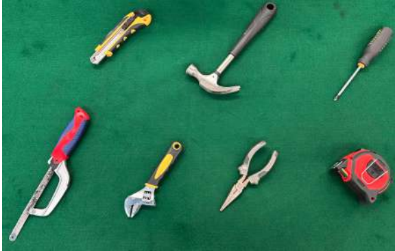
FIGURE 4: Tools used for testing hybrid granular jammer gripper.
