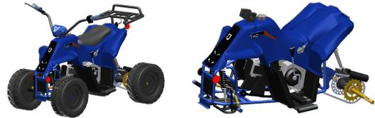
a) Final Expected Assembly of the ATV b) State of the Assembly in Contingency
